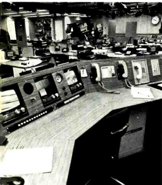
Close-up view of ENC's station in news room. Monitors can show what is coming in over microwave. Two-way radio equipment and phone system to the right. To left, not shown, is more two-way radio gear on 450MHz band. Behind chair is assignment chart, other radio receivers monitoring police bands, etc.
