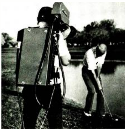
CEI-290 back-pack color TV camera although not designed for news is currently used by WNAC.
